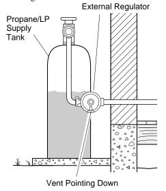
Figure 14 - External Regulator with Vent Pointing Down
